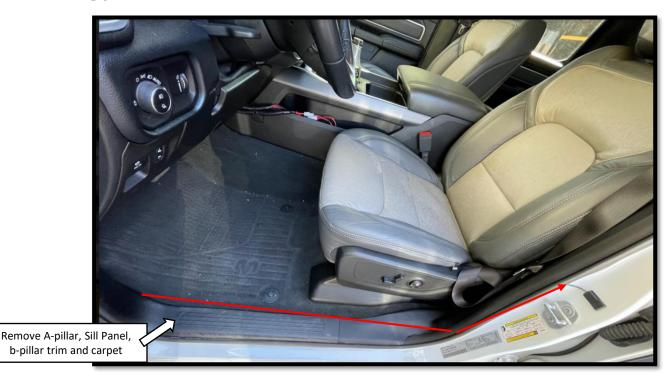
**Step 15:** Route the Driver side door trigger wire (brown) towards the Driver side b-pillar. Route the Passenger side door trigger wire (white) under the center console and over to the Passenger side b-pillar. Route the black disable switch wires to the center console.
