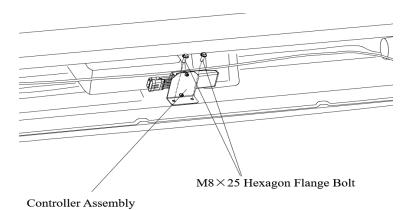
**Step 6**: Locate factorystep mounting hole patternjust below the middle body mount on the driverside of the truck. Remove the tape covering the large slot. Introduce the threaded bracket through the slot and let it hang from the small tab as shown. Install the controller bracket using two M8 flange bolts.
