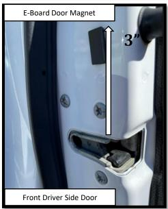
**Step 18:** With the front driver side sensor attached, you can determine the correct position for the door magnet. peel the backing from the double-sided tape and stick the magnet on the door. Align the bottom of the magnet with the 3"
