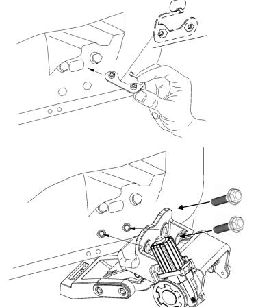
**Step 3**: Install the Front Driver side motor using (1) Nut Plate, (2) M8 Hex Bolts. Holes that do not have factory threaded inserts will require the threaded nut bracket that is included in this kit. The hardware should be hand tightened only until snug. This will allow the motor assembly to move and align easier when installing the running board.
