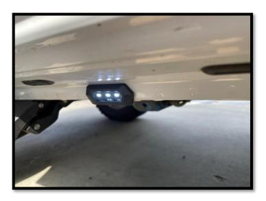
**Step 12**: Align the arrows on the small round connectors and plug the Driver side front and Driver side rear LED lights. Prepare the surface by cleaning with a 50/50 mix of isopropyl alcohol and water or equivalent. Once the surface is completely dry, peel the backing from the double-sided tape and stick the LEDs to the bottom side of the rocker panel. Stick the LED lights at the center of the front and rear Driver side doors
