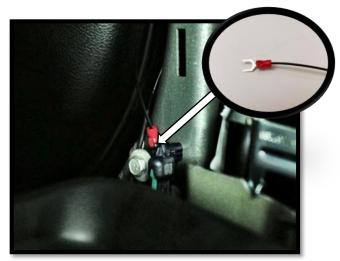
**Step 16:** The door trigger sensor harness will need a ground connection to the vehicle. Locate the hex head screw near the seatbelt assembly and install the ground under the plastic housing as shown.
