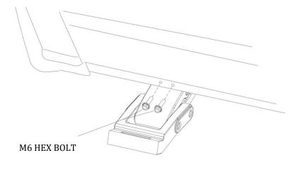
**Step 5**: Install the rear and front Driverside motor using two M6 flange bolts to fasten the motor to the pinch seam. The hardware should be hand tightened only until snug. This will allow the motor assembly to move and align easier when installing the running board.
